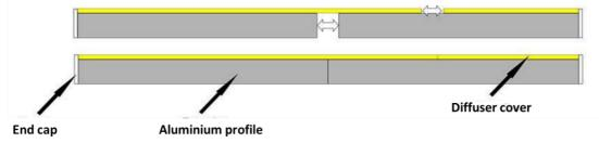
**Tip:** If you are installing multiple profiles in a continuous linear run, it's best to stagger (overlap) the diffuser covers to the aluminium bases. This will mean the joins between the covers are located at different points to the joins between the bases, which will provide a more robust overall solution and look more attractive.
