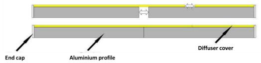
Tip: If you are installing multiple profiles in a continuous linear run, it's best to stagger (overlap) the diffuser covers to the aluminium bases. This will mean the joins between the covers are located at different points to the joins between the bases, which will provide a more robust overall solution and look more attractive.
